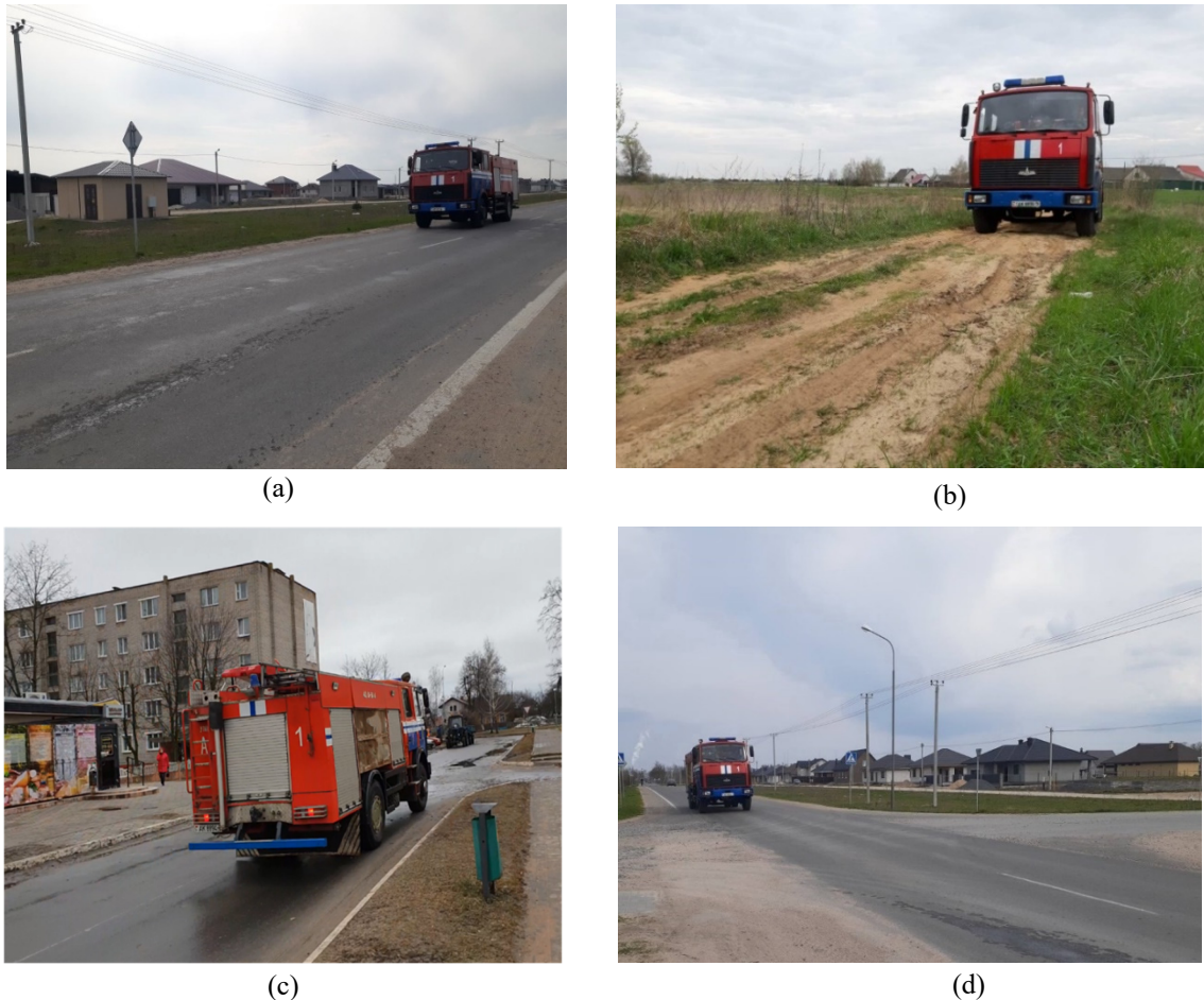
Fig. 5. Investigation of acceleration values arising under the action of inertial loads in the construction of a tank with a volume of 5 m 3 of fire trucks on the MAZ-5337 chassis when driving in mode No. 1 (a); mode No. 2 (b); mode No. 3 (c); mode No. 4 (d)
