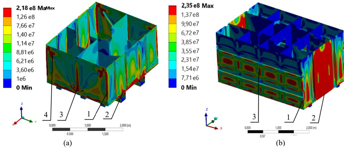
3 – T-joints of breakwaters and walls; 4 – T-joints of stiffeners and side walls
