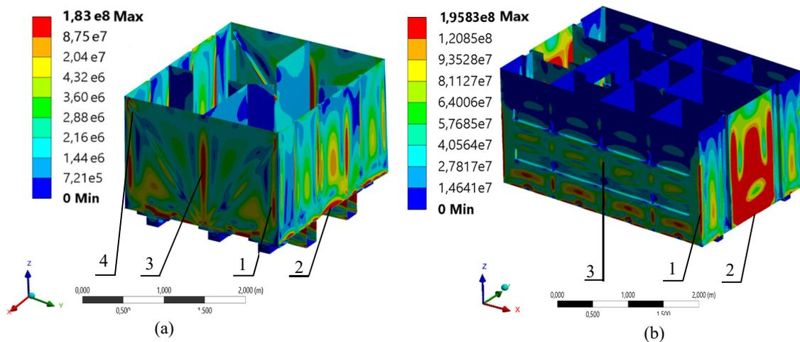
1 – corner joints of the walls; 2 – corner joints of the front, back walls and bottom;
