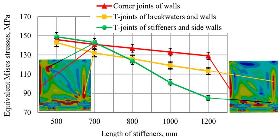
**Fig. 3. The dependences of equivalent stresses arising in the most loaded nodes of a 5 m<sup>3</sup> tank of fire trucks on the MAZ-5337 chassis on the length of the stiffeners in the form of an equilateral angle. The type of stress fields at characteristic points on a fragment of the side wall of the construction**
