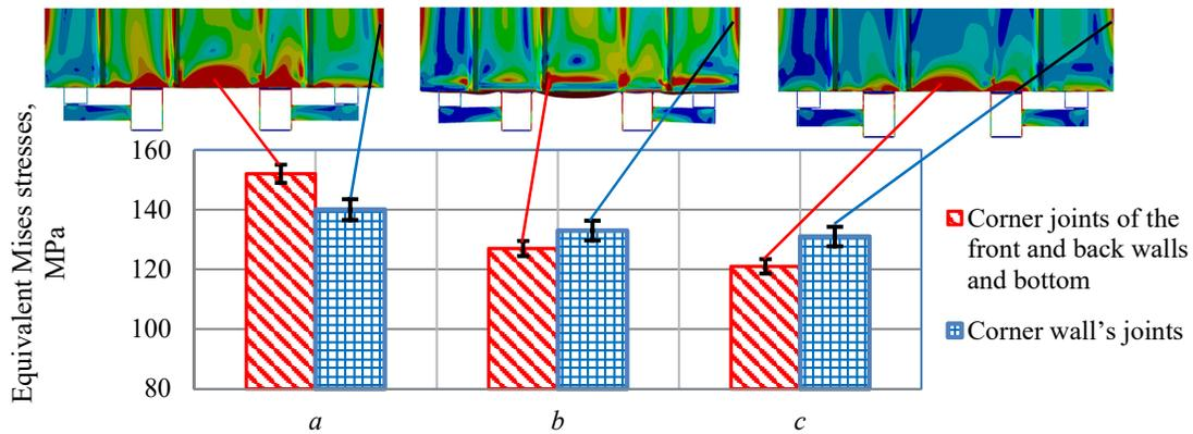
**Fig. 4.** Dependences of equivalent stresses arising in the areas of elements' corner joints of tanks with a volume of 5 m<sup>3</sup> of fire trucks on the MAZ-5337 chassis on the type of their constructions (mass-production (a), upgraded with the installation of corners (b) and profiles U-shaped section (c)) and the type of stress fields at characteristic points on a fragment of the front wall of the construction
