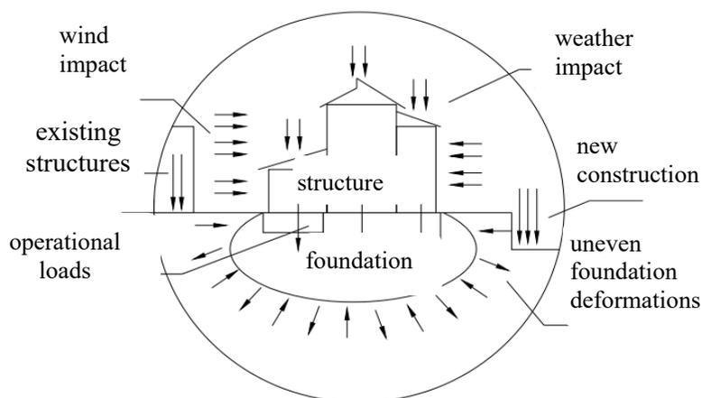
**Fig. 1. Scheme of interaction between the elements of the “foundation – structure” construction system and the environment of the city**
