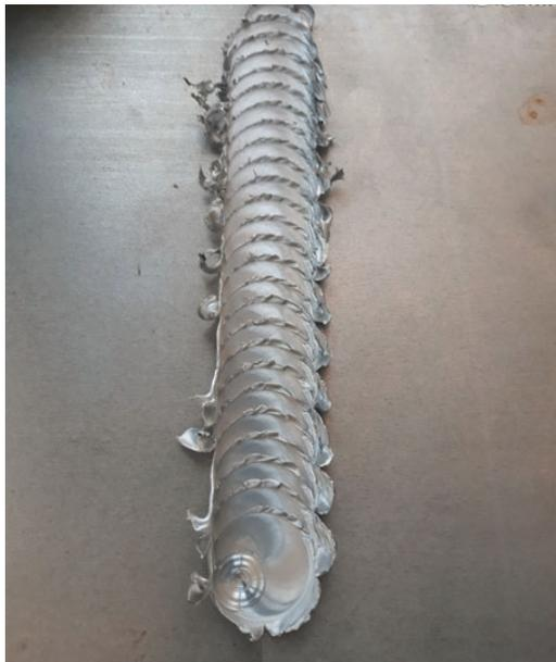
**Fig.5. FSW along cycloid-like trajectory**
