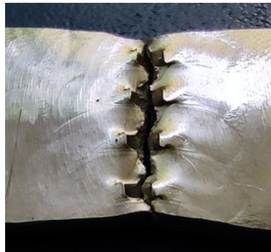
**Fig.13. Fracture of specimen series “S”**
