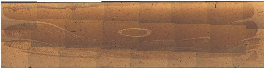
Fig.8. Microstructure image of the weld in FSW along cycloid-like trajectory, series “S”.
