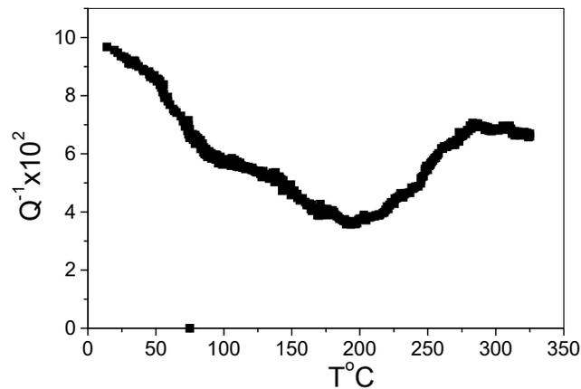
**Fig.3. Temperature dependencies of the internal friction – Micro crystalline specimens after aging (without quenching)**
