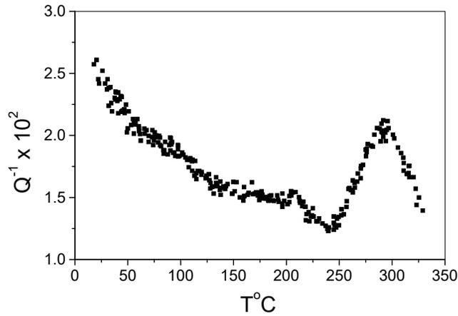
**Fig.2. Temperature dependencies of the internal friction – micro crystalline specimens after quenching and aging**
