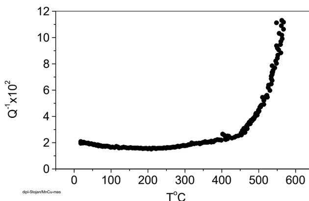
**Fig.1. Temperature dependence of internal friction after quenching and aging of solid specimen**
