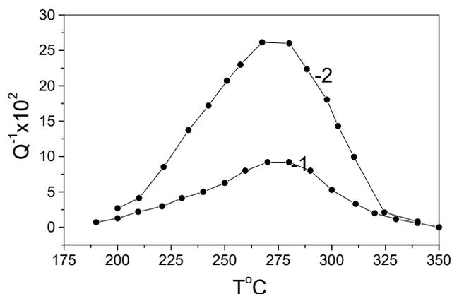
**Fig.4. Internal friction relaxation maximums: 1- after quenching and aging; 2- after aging**
