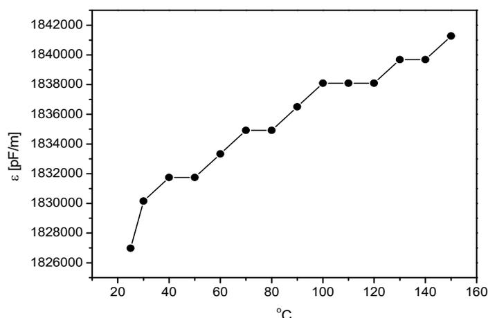
**Fig.2 Dielectric permittivity of SrTiO<sub>3</sub> deposited on an aluminum support**
