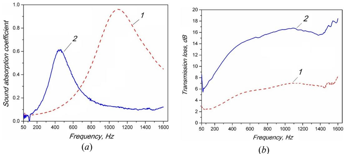
**Fig. 2. Results of measurements of sound absorption (a) and transmission loss (b) of composites based on buckwheat husks and unmodified epoxy resin of various densities: 1 – 500 kg/m<sup>3</sup>; 2 – 700 kg/m<sup>3</sup>(test specimens of 30 mm thick)**
