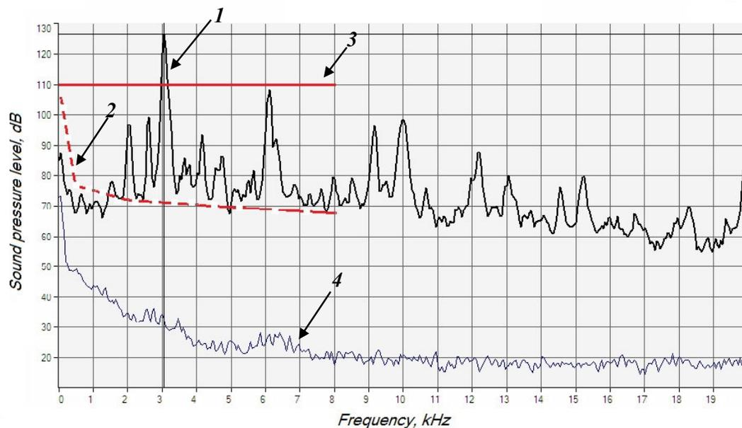
**Fig. 3. Results of measurements of the noise generated during braking of railway carriage with standard brakes: 1 – measured noise levels; 2 – maximum permissible levels (MPL) for constant and equivalent intermittent noise; 3 – MPL for the maximum noise value (110 dB); 4 – background noise level**
