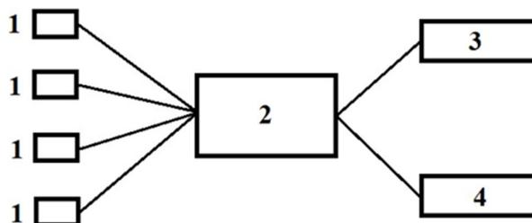
1 – temperature sensors, 2 – logic element, 3 – light alarm, 4 – sound alarm
