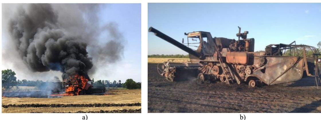
**Fig. 1. – Combine harvester fire (a) and fire consequences (b)**
