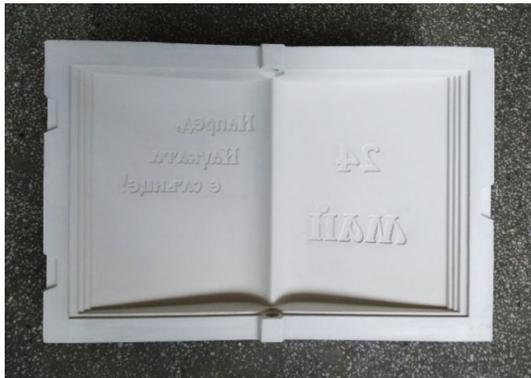
**Fig. 3. First part of plaster of Paris (POP) slip casting mould**
