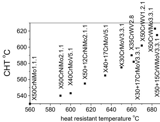
Fig.2. Dependence between a steel heat resistance and CT.
