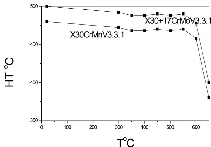
Fig. 3. Variation of CHT of the steel X30CrMoV3.3 and its analogue X30+17CrMoV3.3
