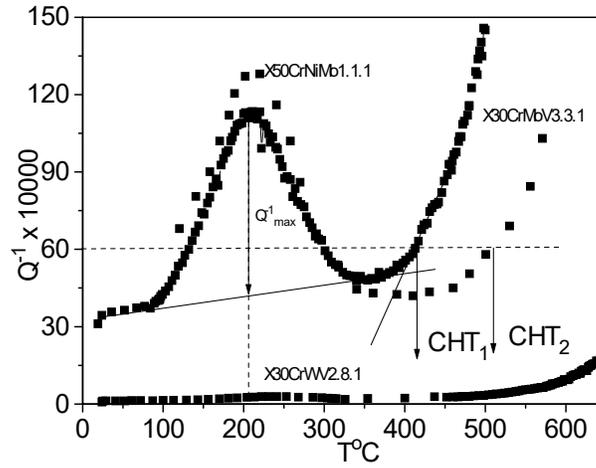
Fig.1. Relaxation spectra of some of the examined carbon hot working steels after quenching
