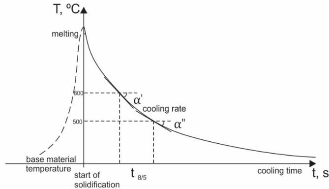
**Fig 1. The cooling rate is a sophisticated function of the process variables (parameters and conditions). In normal conditions the cooling rate at lower temperatures is lower than the cooling rate at higher temperatures,  $\alpha' > \alpha''$ , as a result of the higher temperature gradient  $\Delta T$ .**
