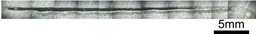
**Fig. 8. Lack of bonding at 65 degrees**
