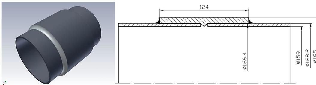
Fig. 1. 3D-view and drawing of experimental samples
