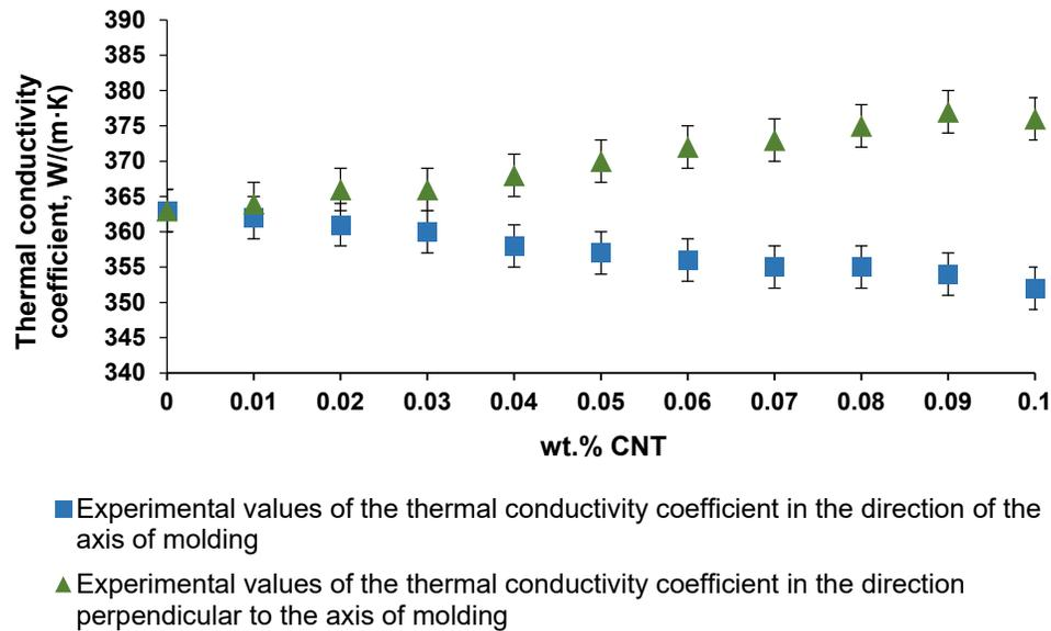
Fig. 1. Thermal conductivity coefficient of the composite materials “copper – CNTs”
