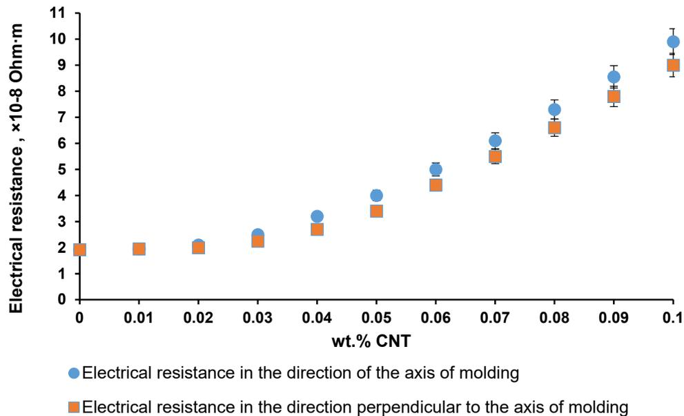
**Fig. 2. Electrical resistance of the composite materials “copper – CNTs”**
