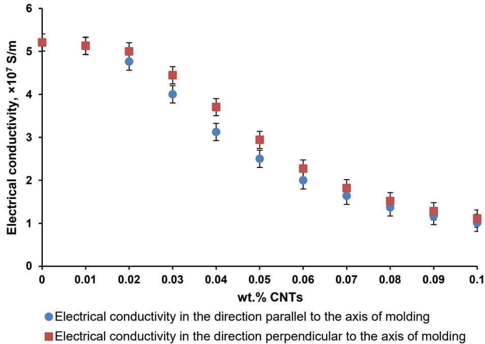
Fig. 3. Electrical conductivity of the composite materials “copper – CNTs”
