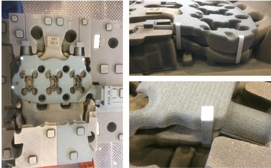
**Fig. 5. Upper and lower core fixing with special aluminum brackets: left – top view; right – side view of the three brackets**
