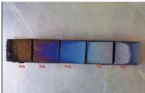
**Figure 5. Image of partial oxidation of the surface of titanium samples coated with glassy carbon at 1350°C**
