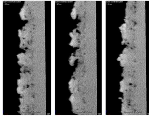
**Figure 3. 3D image of the surface of porous titanium coated with glassy carbon along the xz axis**
