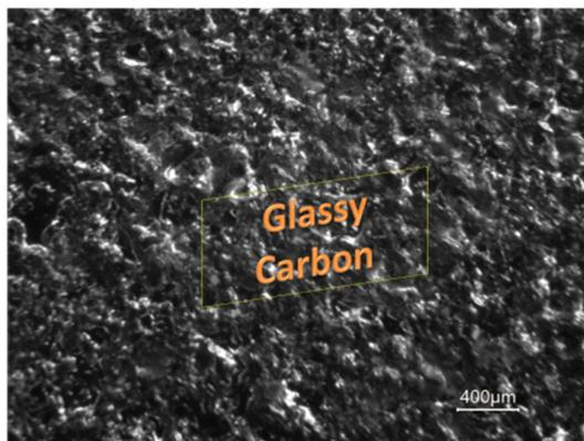
**Figure 1. Micro image of GC coating on titanium sample – x400**
