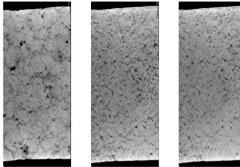
**Figure 4. 3D image of the surface of porous titanium coated with glassy carbon along the yz axis**
