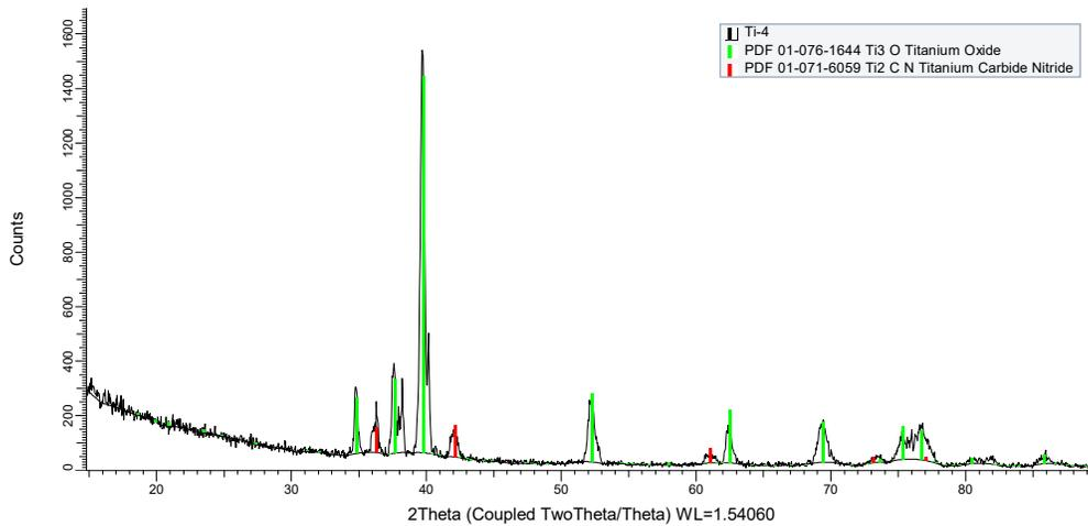
Figure 10. Diffraction pattern of sample Ti4 partially oxidized at 1350°C
