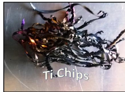
**Figure 6. Image of the partial oxidation of protective titanium chips**
