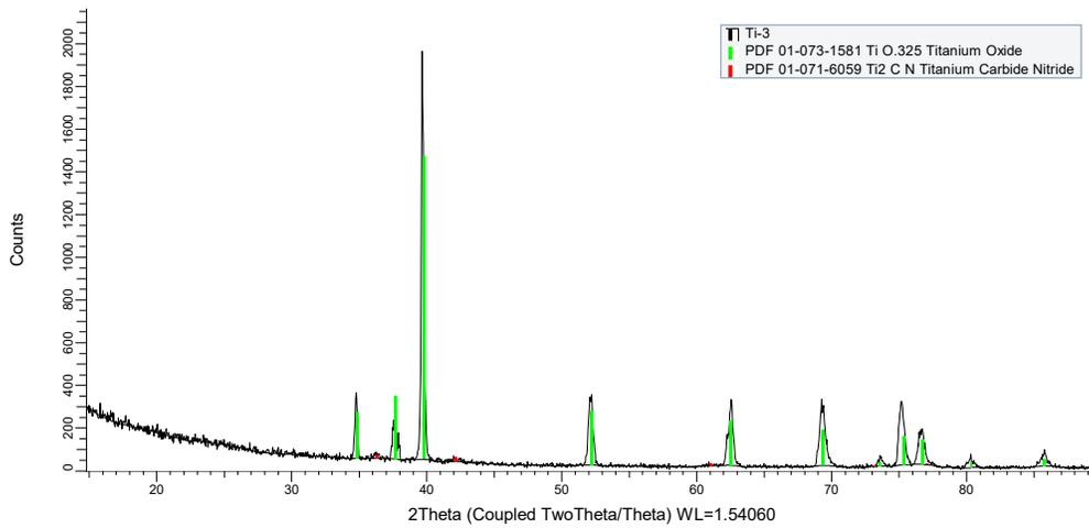
Figure 9. Diffraction pattern of sample Ti3 partially oxidized at 1350°C
