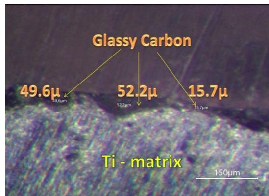
**Figure 1a. Microstructure of GC coating on titanium substrate with porous titanium**
