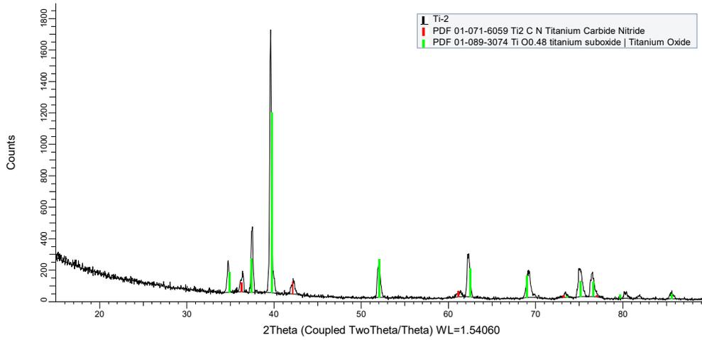
Figure 8. Diffraction pattern of sample Ti2 partially oxidized at 1350°C
