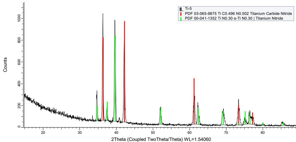
Figure 11. Diffraction pattern of sample Ti5 partially oxidized at 1350°C
