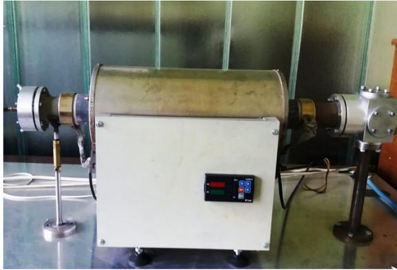
**Fig.2. Tube furnace for thermo-chemical deposition of glassy carbon**
