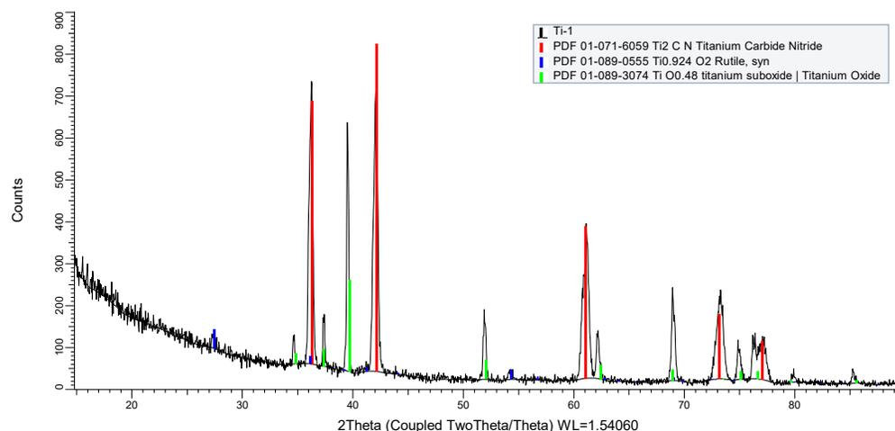
**Figure 7. Diffraction pattern of sample Ti1 partially oxidized at  $1350^\circ\text{C}$**
