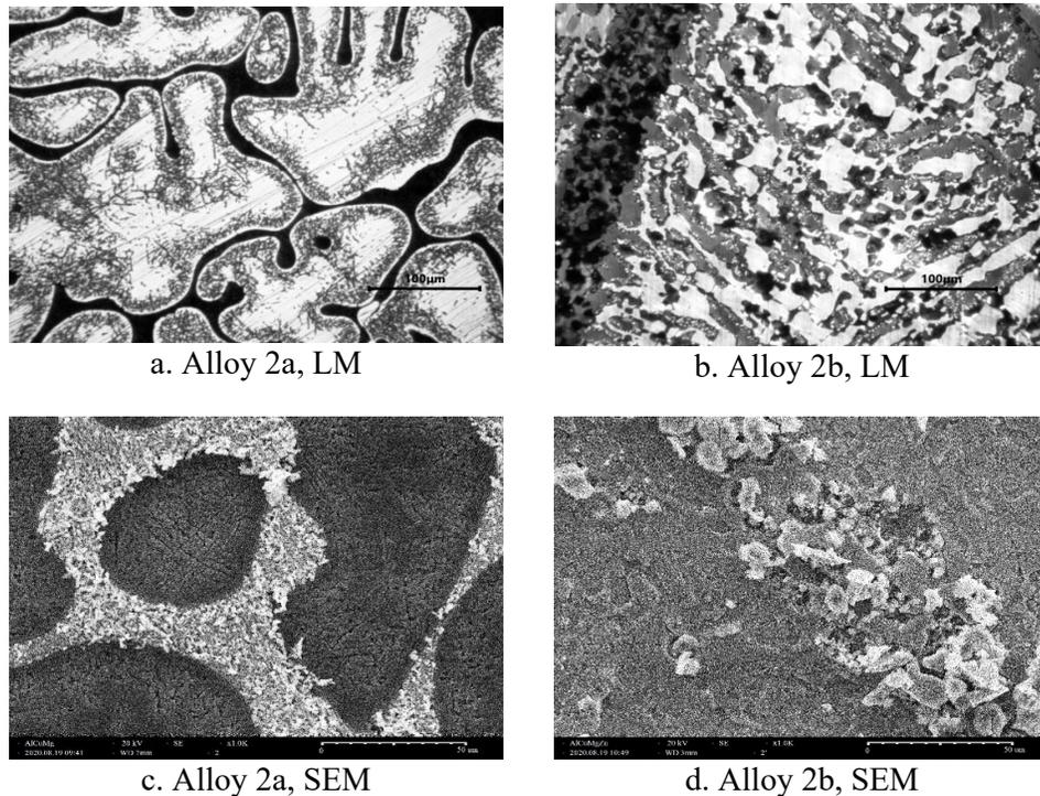
**Figure 3. Microstructure of 2a Al-Cu-Mg and 2b Al-Cu-Mg-Zn alloys**
