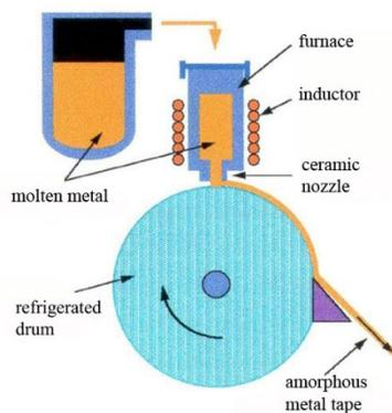
Figure 2. Scheme of PFC equipment.
