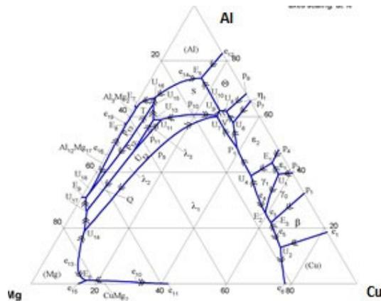
Figure 1. Ternary Al-Cu-Mg diagram
