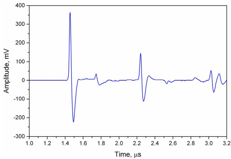
**Fig. 3. Signal measured in 1.5 mm thick shungite I**
