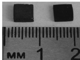
Fig.1. Samples of shungite. The thickness of the left specimen is 1.05 mm, right specimen thickness is 1.5 mm
