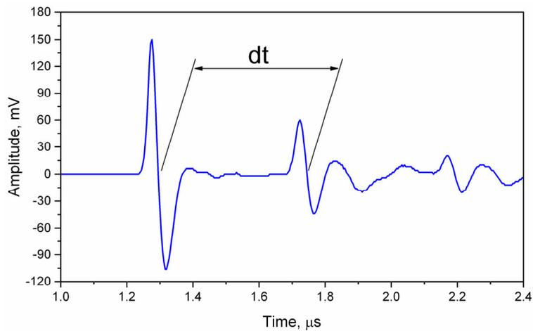
**Fig. 4. Signal measured in 1.05 mm thick shungite II**
