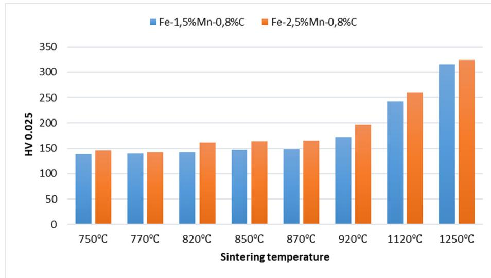
**Fig. 3. Vickers hardness of investigated materials vs. sintering temperature**
