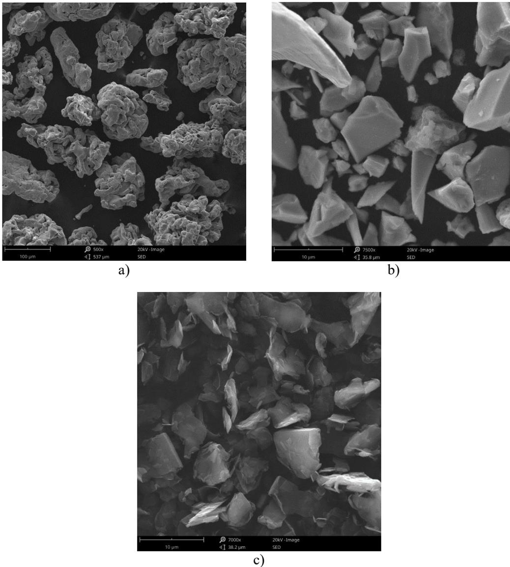
**Fig. 1. The starting powders: a) Höganäs iron powder grade NC 100.24, b) Elkem ferromanganese powder and c) ultra-fine (C-UF) graphite powder**
