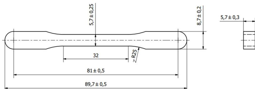
**Fig. 2. Test piece for tensile testing**
