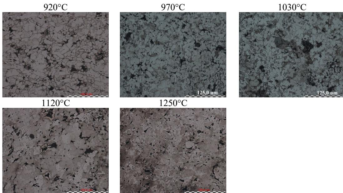
Fig. 5. The microstructure of Fe-1.5%Mn-0.8%C vs. annealing temperature; mag. 200x
