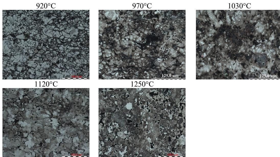
**Fig. 6. The microstructure of Fe-2.5%Mn-0.8%C vs. annealing temperature; mag. 200x**
