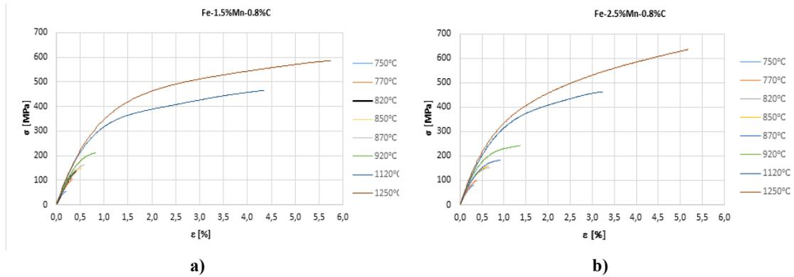
**Fig 4. The effect of sintering temperature on the tensile strength of a) Fe-1.5%Mn-0.8%C and b) Fe-2.5%Mn-0.8%C**
