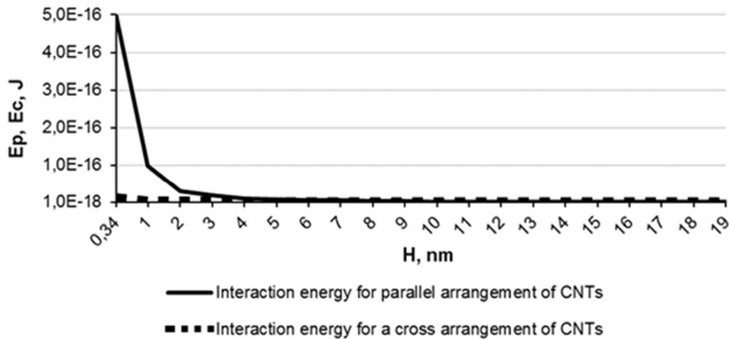
Figure 4. Energy of van der Waals interaction for parallel and cross arrangement of CNTs
