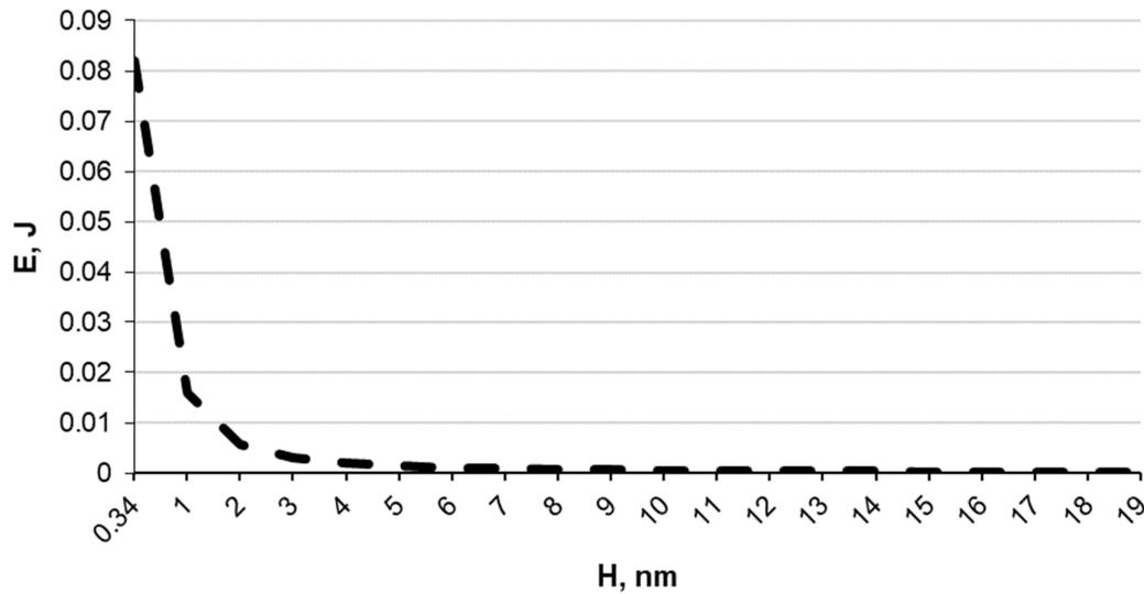
Figure 5. The total energy of van der Waals interaction of CNTs in the agglomerate
