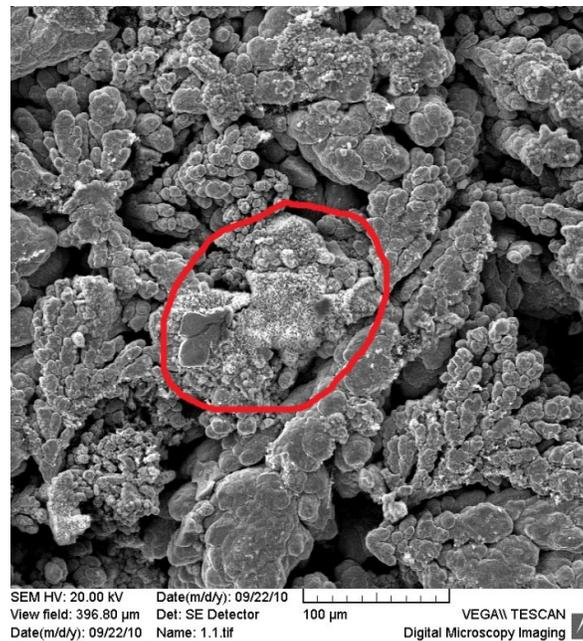
Figure 2. The structure of the metal matrix composition “copper – CNT” with CNT agglomerate
