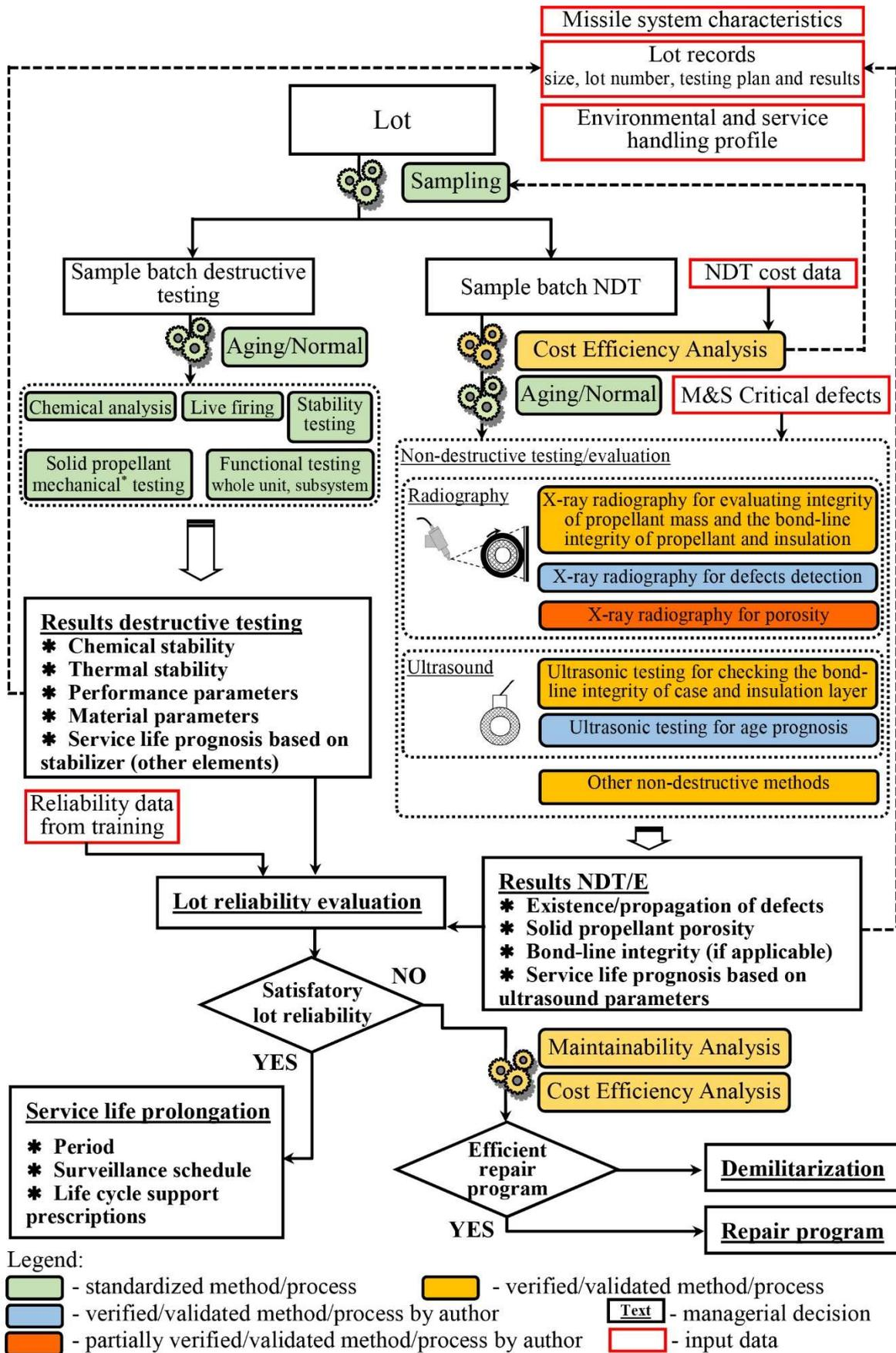
Fig. 5. Comprehensive approach for service life assessment of solid-propellant rocket motors
