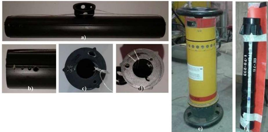
**Fig. 6. Verification testing bet: a) solid propellant; b), c) and d) artificial flows; e) X-ray system; f) sample with X-ray film (Copied from [21])**
