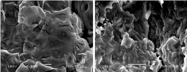
Fig. 4. Micro and macro cracks
