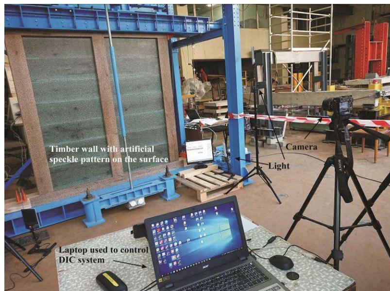
**Fig. 1. Experimental setup with tested timber wall**
