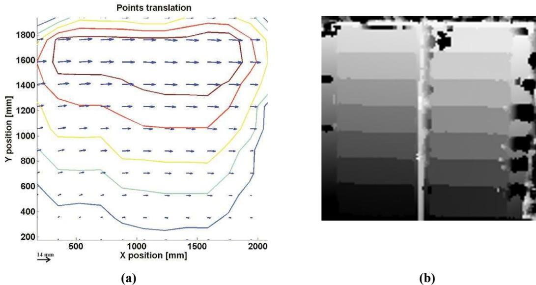
Fig. 4. Horizontal displacement field obtained with DIC: (a) displacement vectors (b) variation of gray
