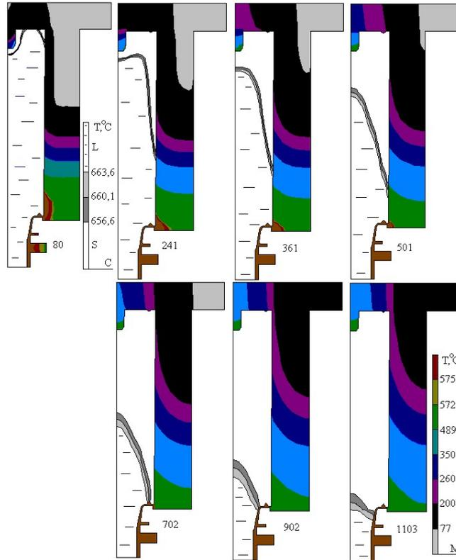
**Fig. 3. Mathematical experiments on the base of mathematical model of the theory of heat conductivity Stefan-Schwartz's 3D problem in physics and engineering Foundry. Initial temperature field is show on (Fig.2 b) and with simple condition  $\alpha_w = \text{const}_w$  at ( $W$ ) and  $\alpha_r = \text{const}_r$  at ( $r$ ) and with condition  $\alpha_w \neq \alpha_r$ . Technological process of solidification is obtained through *the initial temperature field* of the press mold.**
