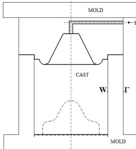
**Fig. 1. General geometric scheme of the gas pressing (GP) method: cylindrical CAST, MOLD and boundaries surfaces W (working) and external  $\Gamma$  (mold/environment); P is pressure [9, 10].**
