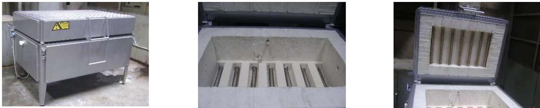
Fig. 2. Pictures of the manufactured and tested "Mida" furnace
