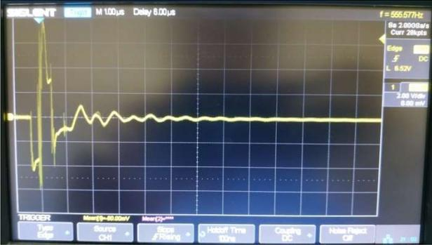
Figure 4. Harmonic oscillations of an ultrasonic transducer with electric damping
