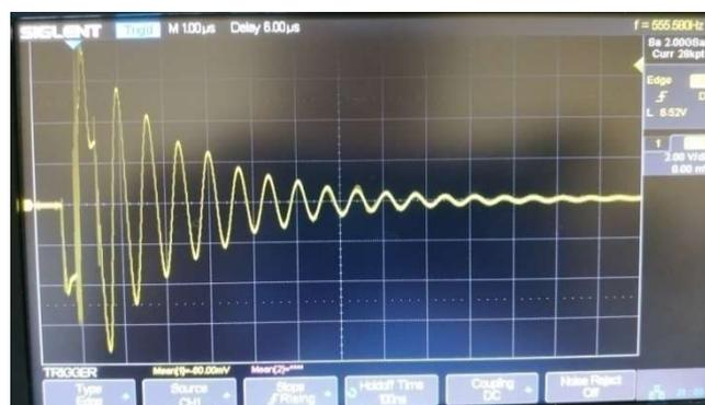
Figure 3. Harmonic oscillations of an ultrasonic transducer without damping
