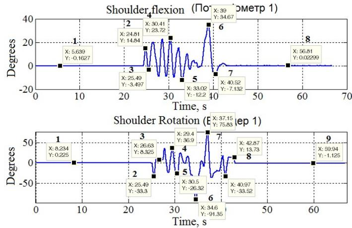
Fig.6. Joint angles of stand-simulator shoulder
