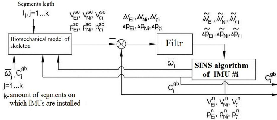
Fig.4 The scheme of data processing in complex algorithm for one IMU of ISEHMP
