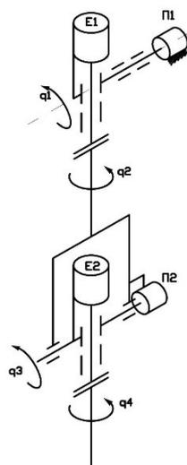
**Fig.5b. Kinematic drawing of upper limb Stand-simulator**
