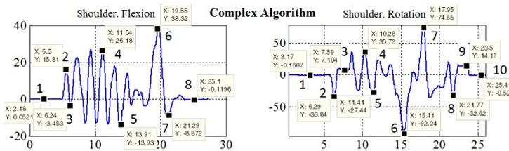
Fig.8 Joint angles of ISEHMP using a complex algorithm
