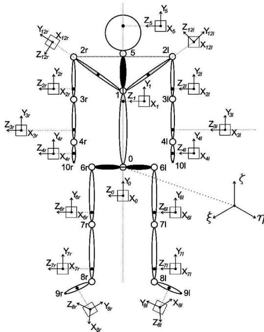
**Fig.1 Biomechanical model of the human body with IMU positions and segment's coordinate systems**
