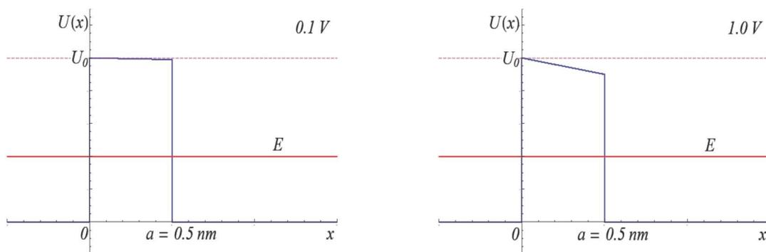
Fig.3. Realistic potential for voltage 0.1 (left) and 1.0 (right) V.
