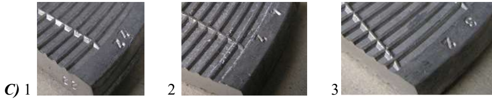
Fig.2 Experimental schema Vacuum in filling of MB-250 and view of cast and surface details [8 and 15]: a) The scheme is executed on a machine MB 250 - the receiver and control valves are mounted on the fixed plate, allowing the shortest distance between the mold and the receiver. For connection is used a special vacuum hose; b) Ripple plate type casting with surface details for pressing abrasive discs standard casting under high pressure [15]; c) Different feeling velocity [8]: 1 – min; 2 – middle; 3 – turbulent.
