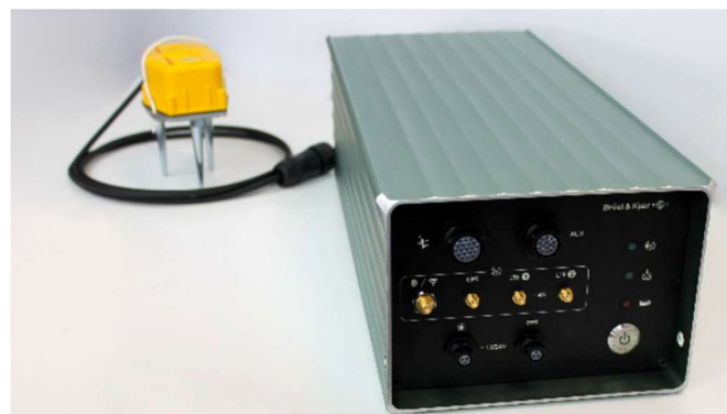
Figure 6. Monitoring logger of seismic and structural vibrations
