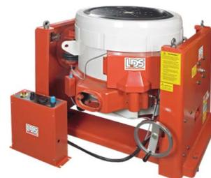
**Figure 5. Type: Air-cooled vibration test system – large**
