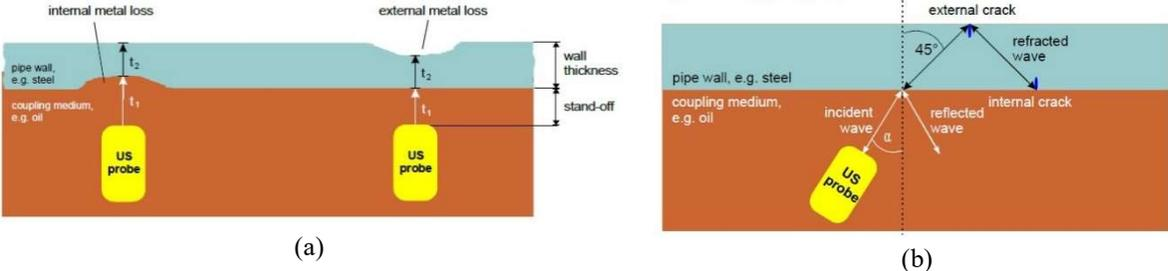
Figure 6. Applied ultrasonic pulse-echo technique to detect deviations in wall thickness (a) and cracks in the wall (b) of pipeline inspected by pipe internal automated system.
