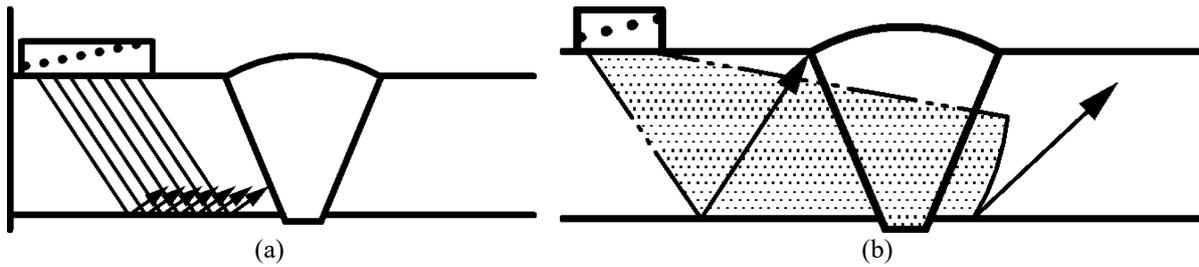
Figure 6. Scheme of electronic scanning with fixed positions of probe: linear (a), sectorial (b), according to EN ISO 13588.
