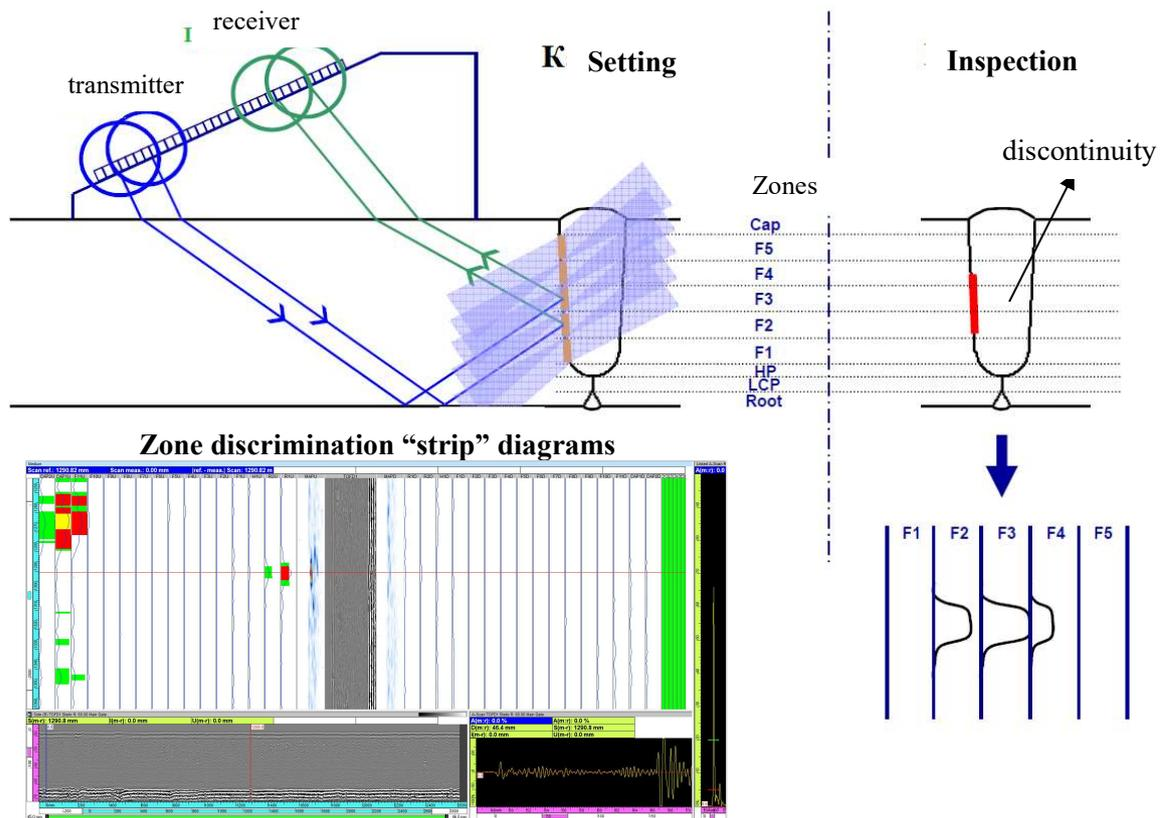
Figure 3. Scheme of inspection and „strip” charts of zone discrimination of weld.
