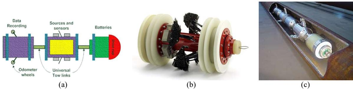
**Photo 3. Schematic diagram of pipe internal automated system (a), scanner head (b) and automated system in a pipe (c).**
