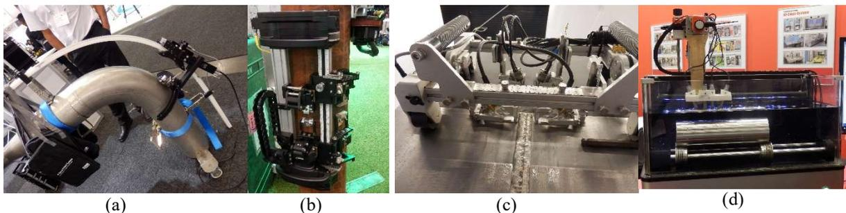
**Photo 2. Mechanised systems: with chain, no magnetic wheels (a), combined with chain and magnetic wheels (b), with magnetic wheels only (c) and immersion bath with mechanised system (d).**
