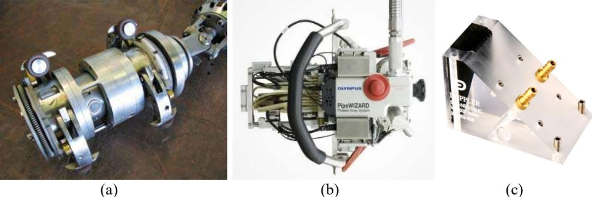
Photo 1. Head of pipe internal (a) and pipe external (b) scanner and wedge (c).
