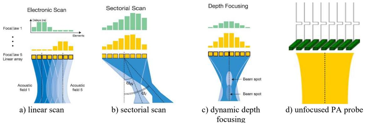
**Figure 1. Types of electronic scanning: linear (a), sectorial (b), dynamic depth focusing (c) and no elements delay set (d) [8].**
