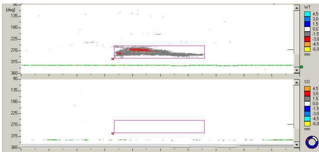
Figure 4. C-scan in pipe internal ultrasonic inspection.
