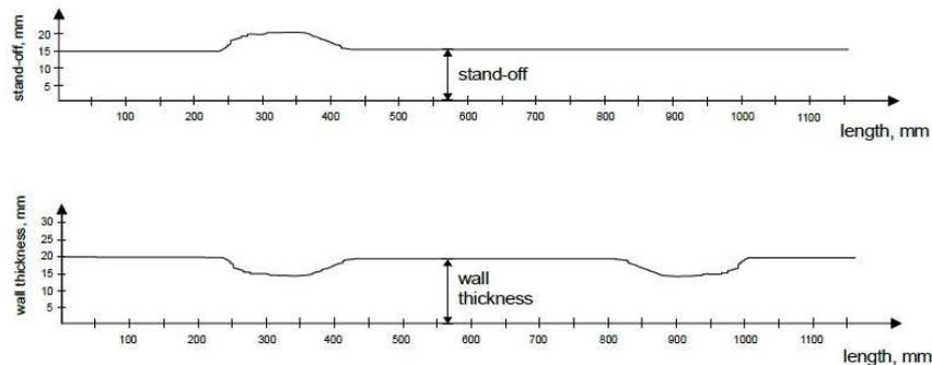
**Figure 5. Principle of ultrasonic determination of wall thickness and B – scan in pipe internal ultrasonic inspection.**
