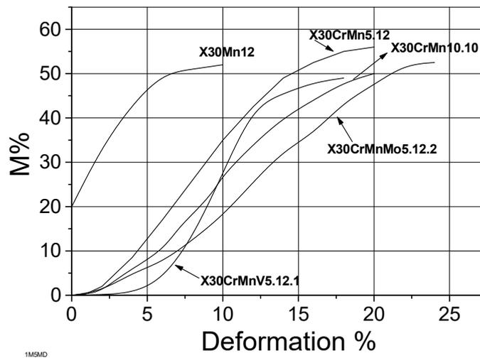
**Fig.1. Dependence of deformation induced martensite quantities in function of the plastic deformation degree**
