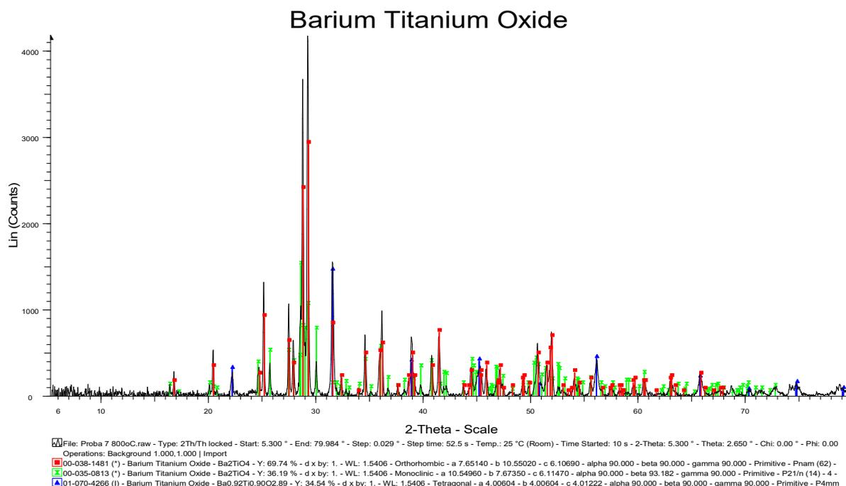
**Fig.2** The phases of  $\text{Ba}_2\text{TiO}_4$  at a temperature  $830^\circ\text{C}$  and retention from 30h.
