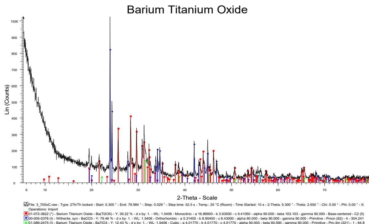
**Fig.1 The phase of BaTiO<sub>3</sub> at a temperature 850°C and retention from 24h.**
