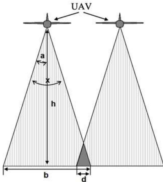
$a$  – the half of the viewing angle of the UAV camera,
