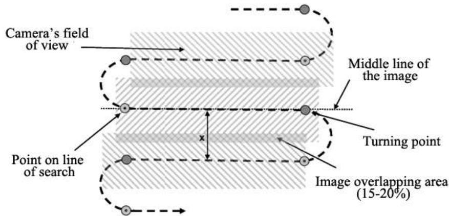
Figure 4. Scheme of flying around a monitoring object using a UAV
