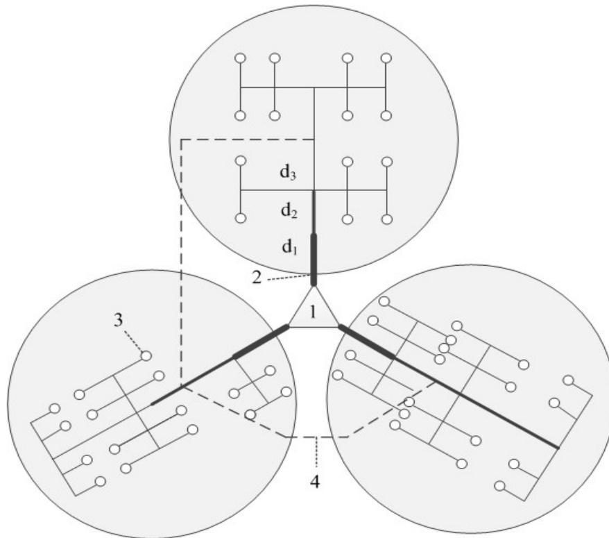
**Figure 1. Structural diagram of radial heat networks:**
