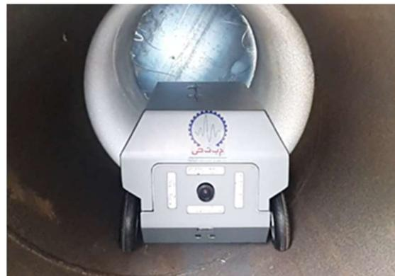
Figure 2. The endoscope "Pipe-Explorer".
